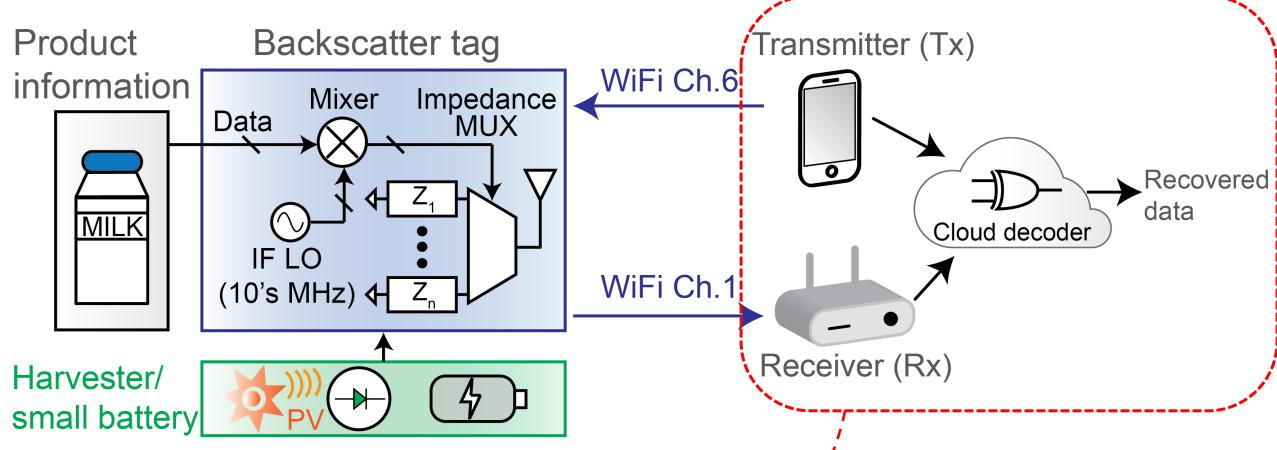
Two access points are required because there are no commercial fullduplex WiFi TRXs, even though Tx and Rx channels are different
