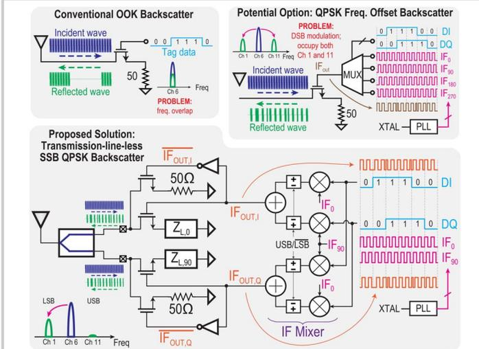
Figure 20.1.3: Methods to perform on-chip backscatter modulation: conventional frequency-overlapped OOK (top left); frequency-offset QPSK (top right); and the proposed transmission-line-less SSB QPSK approach (bottom).
