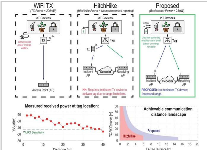
Figure 20.1.1: Proposed WiFi-compliant backscatter approach in contrast to existing art (top); measured RX power at tag location, indicating >30m wake-up range (bottom left); and achievable communication distance landscape.
