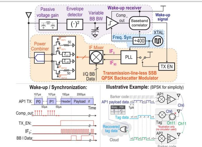
Figure 20.1.2: Block diagram of the proposed backscatter-based IoT tag (top); wake-up/synchronization and backscatter timing (bottom left); BPSK-based example of how tag data is decoded in the cloud (bottom right).
