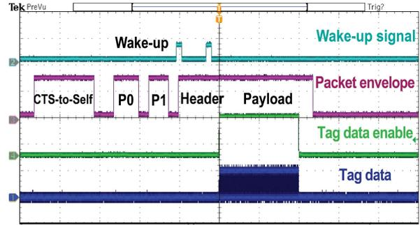
Fig. 13. Measured wake-up and backscatter timing sequence.
