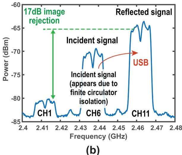
Fig. 12. Measured spectrum showing SSB backscatter-based frequency translation to (a) lower sideband and (b) upper sideband.
