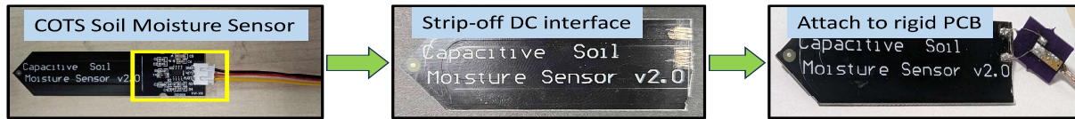
Figure 13: Interfacing a commercial soil moisture sensor:- Step 1: Strip off. Step 2: Small contact pads are etched out to expose copper Step 3: Solder these small leads to rigid impedance profiling PCB.
