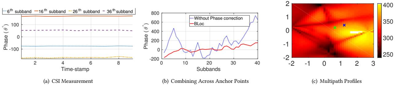
**Figure 8—Microbenchmark:** (a) CSI measurements taken for {6,16,26,36} subbands for 9 instances are constant over time. (b) Phase of without BLoc (Combining over APs) and BLoc (Combining across) for a given client location across subbands, (c) Sample combined Multipath profile in X-Y coordinates, combined across subbands and multiple antennas on an AP and across APs
