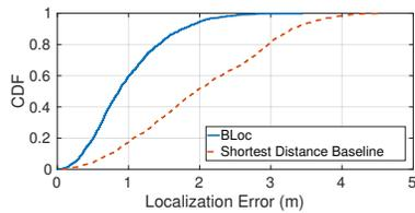
**Figure 12—Effect of Multipath Rejection:** BLoc’s novel multipath rejection scheme improves the accuracy by a factor of 2.
