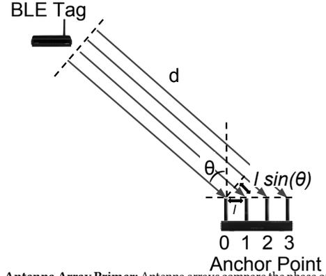
**Figure 2—Antenna Array Primer:** Antenna arrays compare the phase of the received signal at multiple antennas (separated by distance  $l$ ) to identify the angle of the arrival of the signal.
