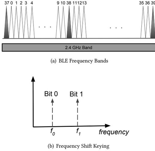
**Figure 1—BLE Primer:** (a) BLE uses 40 frequency bands, 2 MHz wide each, spread over the 2.4 GHz ISM band. Of the 40 bands, 3 are designated advertisement bands (shaded) and the other 37 are data communication bands. (b) BLE uses Gaussian Frequency Shift Keying modulation where each bit corresponds to a different frequency.
