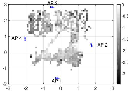
**Figure 13—Correlation of accuracy with Location:** BLoc’s accuracy variation with the location of the BLE tag across the environmental setup.
