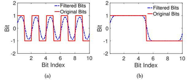
**Figure 4—GFSK:** (a) Gaussian filter applied to random BLE data leads to smooth changes in bits, but consequentially means that the frequency of the transmission is never static. (b) BLoc batches together long sequence of bits to ensure that a stable frequency is reached to obtain meaningful phase and amplitude measurements.
