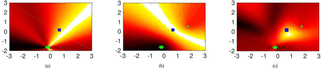
**Figure 6—CSI to Location:** (a) The likelihood distribution of a signal source obtained using multiple antennas on a single anchor point using Eq. 15, (b) The likelihood distribution of a signal source obtained using multiple frequency bands using Eq. 16. The shape of the high likelihood region is hyperbolic because the distances measured are relative. (c) The combined likelihood distribution obtained using Eq. 17. Blue square marks the actual location of the source.
