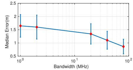
**Figure 10—Effect of Bandwidth:** Shows how the median localization error for BLoc varies with increasing the possible bandwidth of hops for BLE
