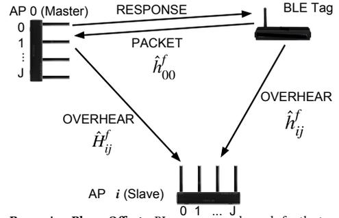
**Figure 5—Removing Phase Offsets:** BLoc measures channels for the two-way communication at the slave anchor’s (AP  $i$ ’s) first antenna ( $j=0$ ),  $\hat{h}_{ij}^f$ , from the BLE tag to the master anchor (AP0),  $\hat{h}_{ij}^f$  and the master anchor to the target,  $\hat{h}_{00}^f$ . It then combines these measurements as shown in Eq. 10 to remove phase offsets.
