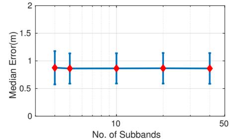
**Figure 11—Interference Avoidance:** Shows how the median localization error for BLoc varies with limiting the number of possible available subcarriers without contention over 80MHz bandwidth for BLE
