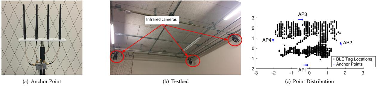
**Figure 7—Implementation:** (a) A shot of one of the 4 antenna Anchor points of the setup, (b) The infrared camera to measure the ground truth for calculating localization errors, (c) The top-view of the setup, we have 4 Anchors with 4 antenna each (in blue +) and the 1700 ground truth positoins of the BLE tag.
