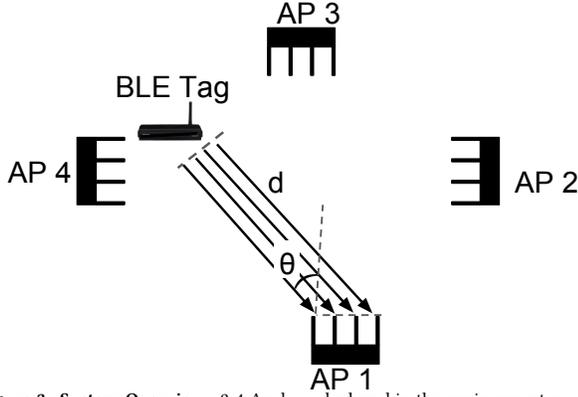
**Figure 3—System Overview:** 2-4 Anchors deployed in the environment measure phase and amplitude of the target tag’s signal received at multiple antennas. These channels are then processed to give information about distance and angle, which is further mapped over 2D space to identify the location of the target devices.
