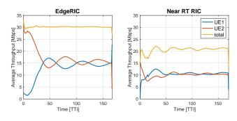
Figure 8: CQI-Fair Allocation with 2UE synthetic channels - one can support higher throughput while maintaining the stability of backlog buffers
