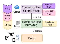
Figure 1: Timescales of RAN Intelligent Control for O-RAN. We desire realtime control at a latency < 1 ms.
