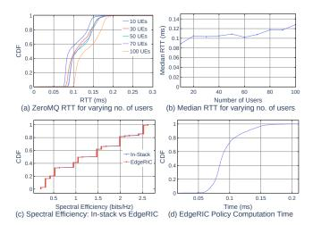
Figure 4: EdgeRIC Feedback latency, spectral efficiency and AI-policy execution times.
