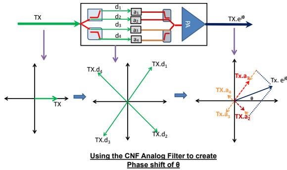
Figure 10: FF's constructive analog filter. The filter enables us to rotate the input signal TX by a fixed angle  $\theta$  by appropriately adjusting the gains on the four taps of the analog filter. The four taps are placed 90 degrees apart, which at 2.45GHz implies that the tap delays are in increasing multiples of 100 picoseconds.
