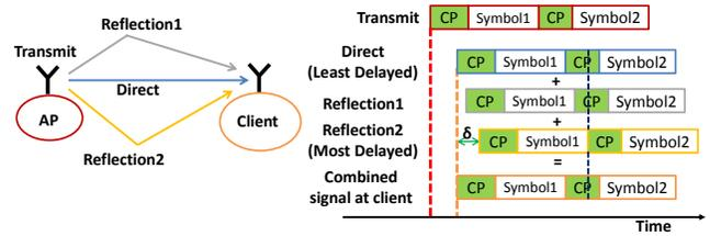
OFDM is resilient to multipath reflections as long as the most delayed reflection is still within the CP of the least delayed component of the same symbol
