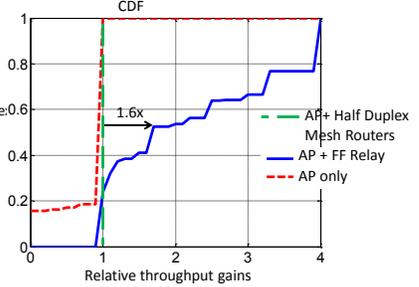
Figure 14: FF’s throughput gains due to SNR amplification from construct-and-forward relaying for a SISO AP, FF relay and client. FF provides a median gain if  $1.6\times$  even without the benefit of MIMO rank expansion.
