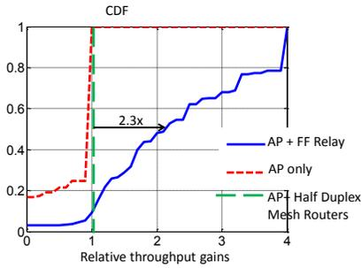
Figure 12: FF’s overall throughput gains. FF provides a  $3\times$  increase in median throughput, and nearly a  $4\times$  gain in dead spot scenarios. Further, it significantly outperforms half duplex mesh routers, almost by a factor of  $2.3\times$ .
