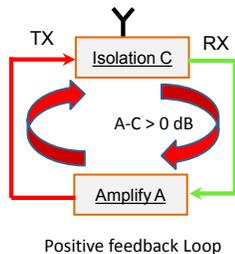
Figure 7: Amplification  $A$  is limited by the amount of isolation  $C$ . Amplifying more than the isolation implies there is still some residual left over after isolation by  $C$  dB, which is then again amplified and relayed in the next time instant and so on. This creates an unstable positive feedback loop.
