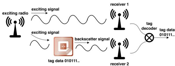
**Figure 1: FreeRider system overview. An example scenario could be office setting where our smart-phone can act as exciting radio, and the WiFi APs as receiver 1 and receiver 2. The WiFi APs are connected by Ethernet backhaul which performs the decoding operation and sends tag data to the Internet.**
