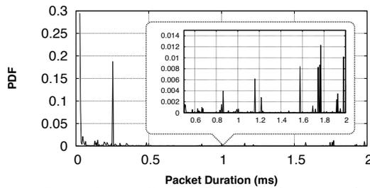
**Figure 3: Durations of 30 million packets on ch. 6 collected in a lecture hall. We see a bimodal distribution where  $\sim 78\%$  of packets last less than  $500\mu\text{s}$  and  $\sim 18\%$  last  $1500\mu\text{s}$ - $2700\mu\text{s}$ . With a pulse-width error bound of  $25\mu\text{s}$ , the probability an ambient packet having the same length as our pulses is about  $0.03\%$ .**
