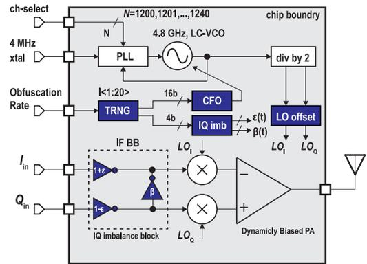
Fig. 3. Privacy enabled WiFi/BLE Tx with integrated TRNG and VCO obfuscation circuit.
