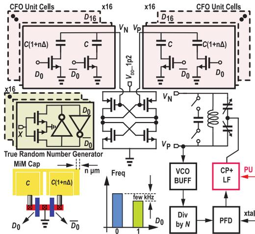
Fig. 4. CFO implementation by using semi-identical MIM caps.
