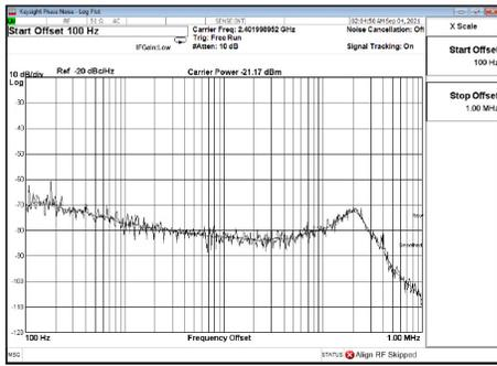
Fig. 7. Measured phase noise of the advertising channel-37 of BLE, with  $-110$  dBc/Hz spot noise at 1 MHz offset and 0.1m rad IPN (100Hz to 1MHz).
