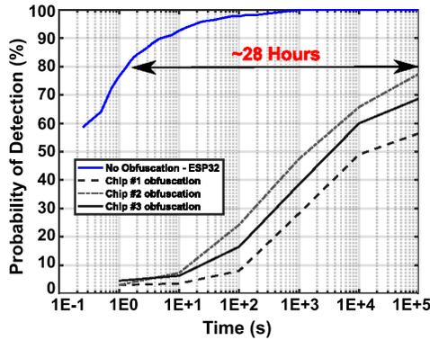
Fig. 8. Obfuscation comparison using the proposed chip (measured chip performances) compared with COTS Tx.
