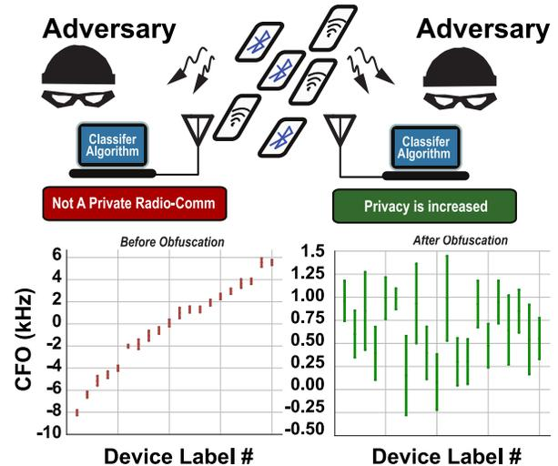
Fig. 1. (a)  $[\mu - \sigma, \mu + \sigma]$  of CFO data measured across hundreds of packets from 20 separate ESP32 BLE chipsets, showing unique and identifiable CFOs. (b) Theoretical data for CFO obfuscation, illustrating that unique identification is much more difficult.
