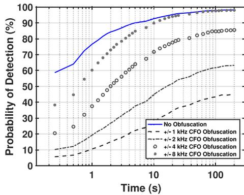
Fig. 2. The effect of CFO obfuscation method on attacker’s ability to identify the BLE devices for different LSB values (1, 2, 4, 8 kHz) when 32 CFO states are available (5 bits).
