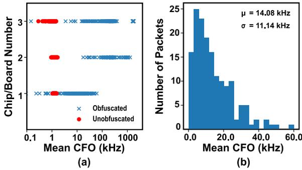
Fig. 6. Measured TRNG enabled, (a) mean frequency CFO and (b) the histogram while transmitting BLE packets (for chip/board #1).
