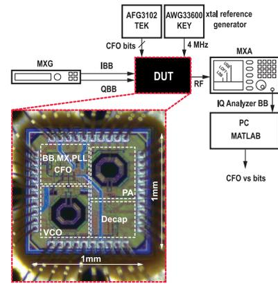
Fig. 5. Measurement setup and die photograph of the private BLE Tx.
